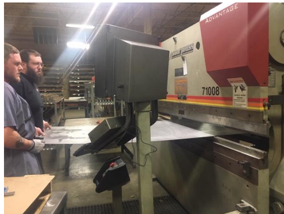
Using Teamwork to CNC Form the laser cut components.
